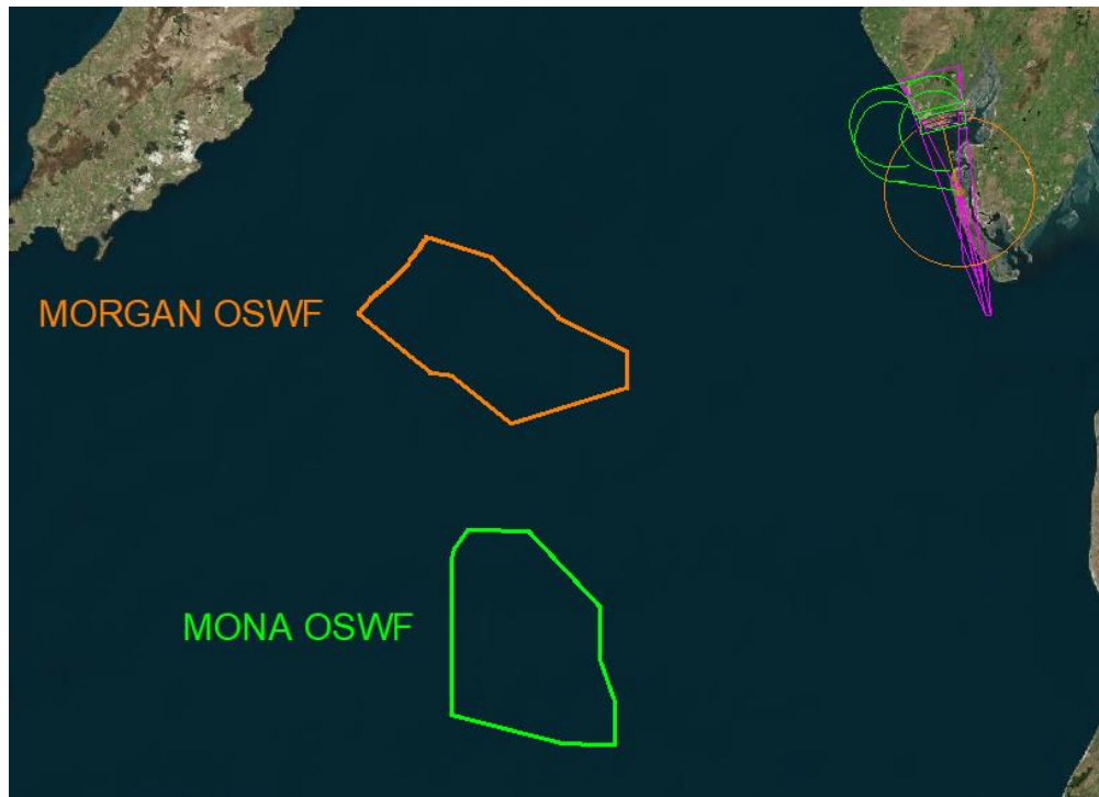
Figure 225 - Morgan and Mona Windfarm vs ILS/DME RWY 35 Protection Areas
