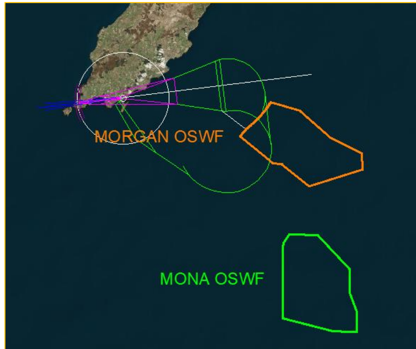
Figure 118 - Morgan and Mona Windfarm vs OFFSET ILS/DME RWY 08 Protection Areas
