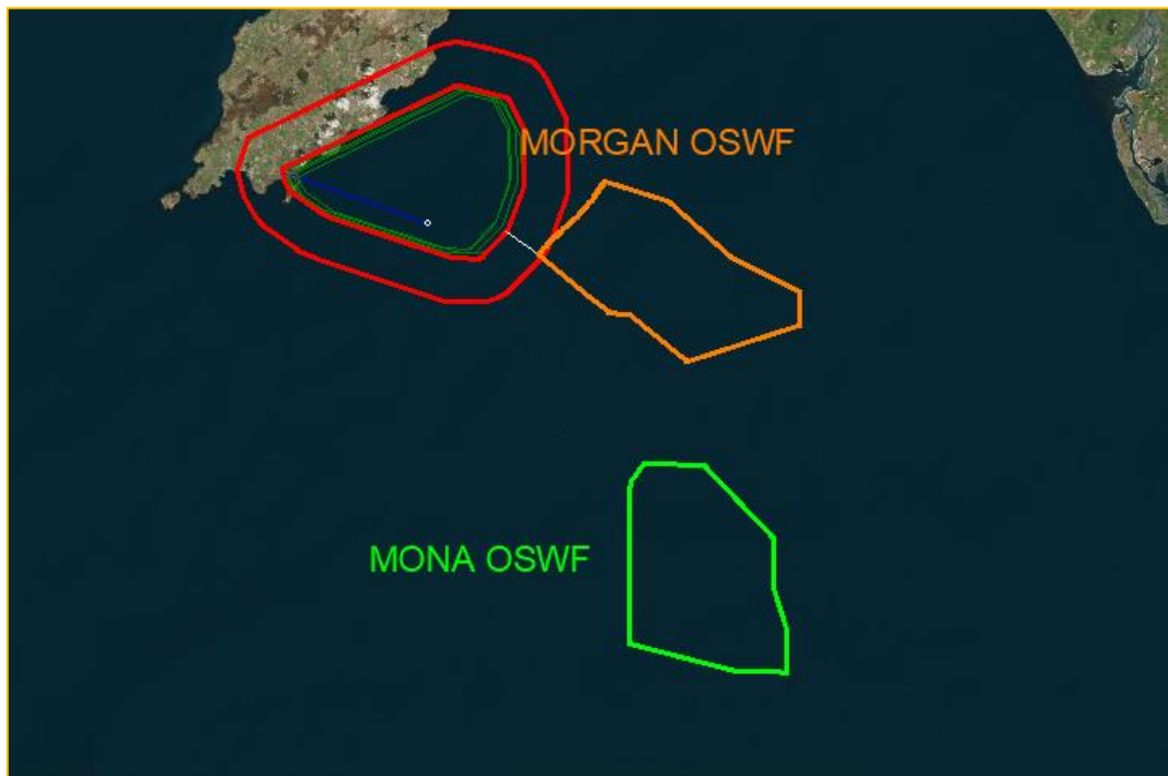
Figure 136 - Windfarms vs ILS/DME RWY 26 Base turn CAT C,D
