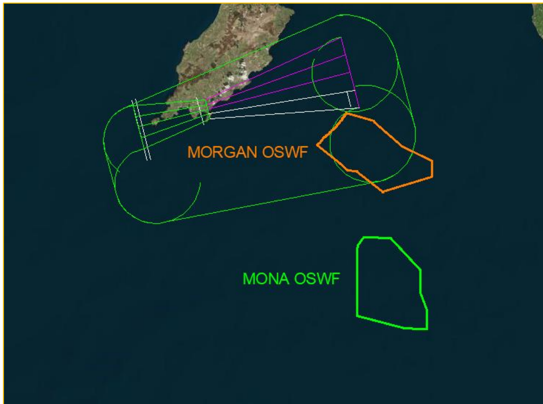
Figure 145 - Morgan and Mona Windfarm vs NDB(L)/DME RWY 26 (NO DME) Protection Areas
