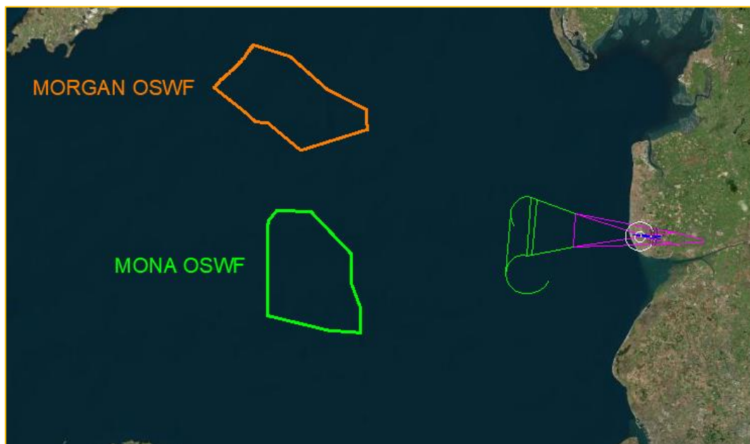
Figure 208 - Morgan and Mona Windfarm vs LOC/DME RWY 28 Protection Areas
